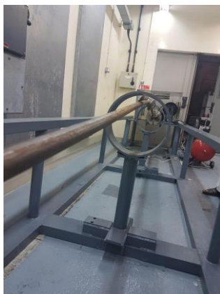
Fig. 18. Large lateral amplitude for 1" drill string near its rotational critical speed.
