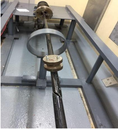
Fig. 23. Fatigue failure of 1" drill string
